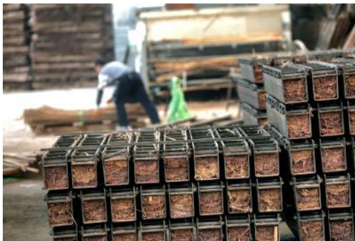
Figure 5: Strand Woven Bamboo beams are made by compressing rough bamboo fibres in moulds under very high pressure (photos MOSO International)
